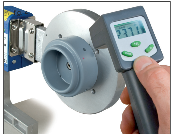
Checking of the temperature with a surface temperature measuring instrument.
